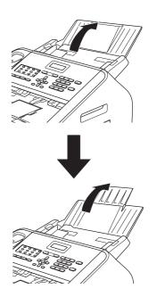
Open the control panel cover by lifting it toward the back.
