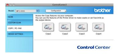
To use the **Copy** buttons, configure the printer driver by clicking the button while holding down the **Ctrl** key.
