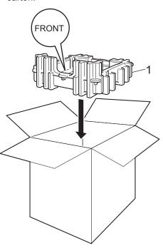
Wrap the machine in a plastic bag, then put it on the bottom packing material (1).
