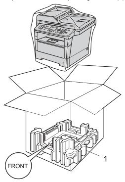
but the two packing material pieces (1) into the carton matching the right of the machine to the "RIGHT" mark on one of the packing material pieces, and the left of the machine to the "LEFT" mark on the other packing material piece. Put the AC power cord and printed materials in the original carton as shown in the illustration.
