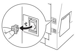
Connect the network interface cable to the Ethernet port and then connect it to a free port on your hub.
