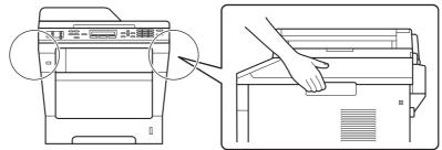
• If you use a Lower Tray, DO NOT carry the machine with the Lower Tray as you may be injured or cause damage to the machine because it is not attached to the Lower Tray.
