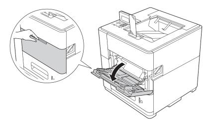
2 Pull out the MP tray support (1) and unfold the flap (2).
