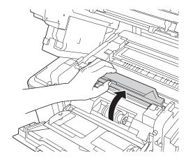
10 Wipe the pick-up roller (1) inside of the machine to remove dust.
