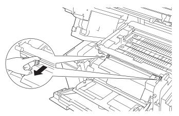
6 Hold the left and right edges of the jammed paper near the inside of the machine and pull it out.
