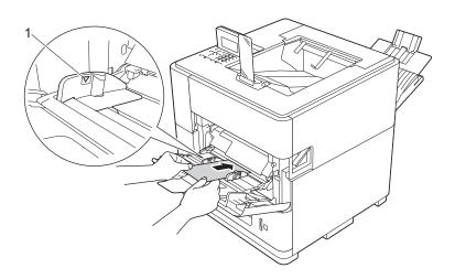
6 While pressing the gray paper-guide release lever (1), slide the paper guide to fit the paper size.
