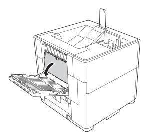
3 Using both hands, gently pull the jammed paper out of the back of the machine.
