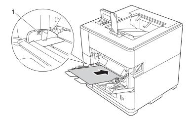
4 While pressing the gray paper-guide release lever (1), slide the paper guide to fit the paper size.
