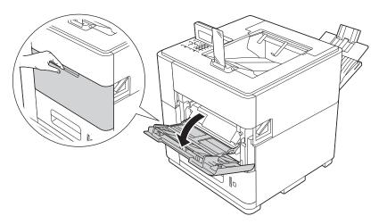
4 Pull out the MP tray support (1) and unfold the flap (2).
