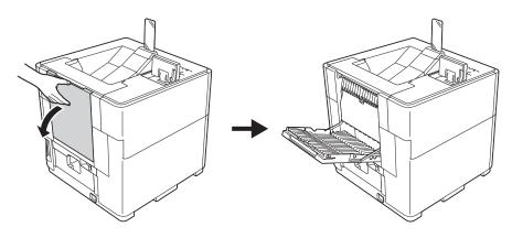
2 Pull out the face-up output tray support (1) and unfold the flap (2).
