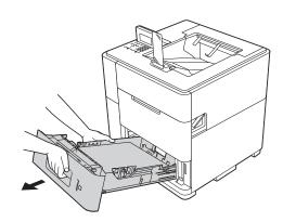
9 Make sure that the jammed paper does not remain under the machine from static electricity.
