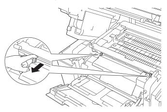
5 Slowly pull the paper tray out until it stops. Then slightly lift the front of the tray and pull the tray out of the machine.
