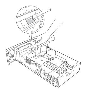
5 Wipe the two pick-up rollers (1) inside of the machine to remove dust.
