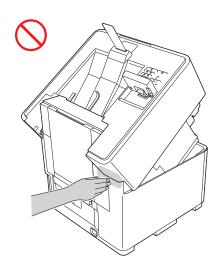
This machine is heavy and weighs more than 40 kg. To prevent possible injuries at least two people should lift the machine by holding it from the front and back. Be careful with the output stopper when moving or lifting the machine. There is a risk of injury if your face or body strikes the output stopper. Be careful not to pinch your fingers when you set the machine back down.
