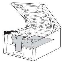
Remove the orange packing piece from each drum and toner cartridge assembly.
