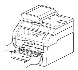
4 Use both hands to push one sheet of paper *firmly* into the manual feed slot until the top edge of the paper presses against the paper feed rollers. Continue pressing the paper against the rollers for about two seconds, or until the machine grabs the paper and pulls it in further.
