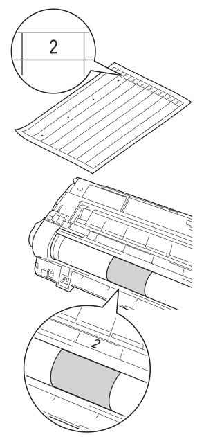
Turn the edge of the drum unit toward you by hand while looking at the surface of the suspected area.
