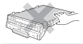
5 Unpack the new belt unit and put the new belt unit in the machine.
