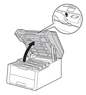
3 Remove the toner cartridge and drum unit assembly for the colour shown on the Touchscreen.
