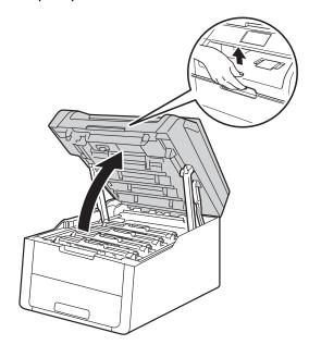
2 Remove the toner cartridge and drum unit assembly.
