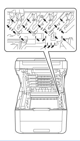
3 Clean the corona wire inside the drum unit by gently sliding the green tab from left to right and right to left several times.
