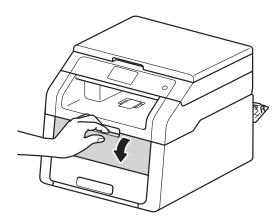
4 Use both hands to slide the manual feed slot paper guides to the width of the paper that you are going to use.
