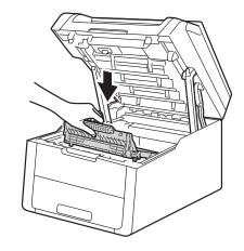
Slide each toner cartridge and drum unit assembly into the machine, making sure you match the toner cartridge colours to the same colour labels on the machine.
