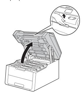
3 Remove all of the toner cartridge and drum unit assemblies.
