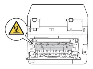
3 Pull the green tabs at the left and right sides down to release the fuser cover (1).
