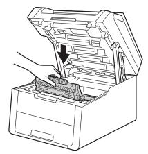
6 Slide each toner cartridge and drum unit assembly into the machine, making sure you match the toner cartridge colours to the same colour labels on the machine.
