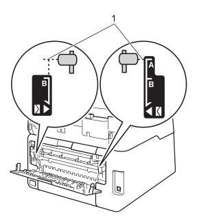
■ Identify the colour causing the problem and install a new drum unit (see *Replacing the drum units* on page 53).
