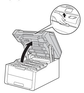
Remove the toner cartridge and drum unit assembly for the colour shown on the Touchscreen.
