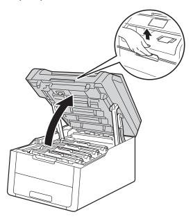
11 The colour of printed dots is the colour of the drum you should clean. Remove the toner cartridge and drum unit assembly of the colour causing the problem.
