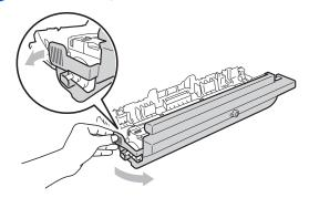
Put the toner cartridge firmly into the new drum unit until you hear it lock into place. If you put the cartridge in correctly, the green lock lever will lift automatically.
