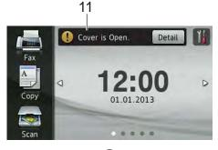
The warning icon papears when there is an error or maintenance message; press Detail to view it, and then press to return to Ready mode.
