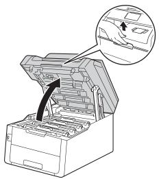
12 The color of printed dots is the color of the drum you should clean. Remove the toner cartridge and drum unit assembly of the color causing the problem.
