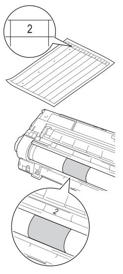
17 Turn the edge of the drum unit toward you by hand while looking at the surface of the suspected area.
