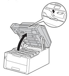
Remove the toner cartridge and drum unit assembly.
