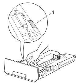
5 Wipe the two pick-up rollers (1) inside the machine to remove dust.
