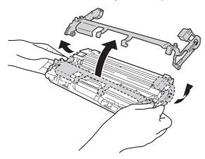
**G** Using both hands, hold each drum and toner cartridge assembly level, and gently shake it from side to side several times to distribute the toner evenly inside the assembly.
