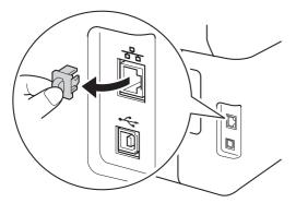
C Connect the network interface cable to the Ethernet port on your machine, and then connect it to a free port on your hub.
