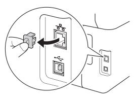
C Connect the network interface cable to the Ethernet port on your machine, and then connect it to a free port on your hub.
