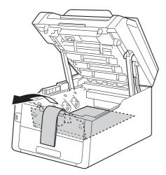
Remove the orange packing piece from each drum and toner cartridge assembly.
