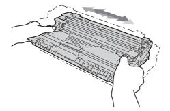
Slide all four drum and toner cartridge assemblies into the machine. Make sure the toner cartridge colour matches the same colour label on the machine.
