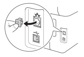
Connect the network interface cable to the Ethernet port on your machine, and then connect it to a free port on your hub.
