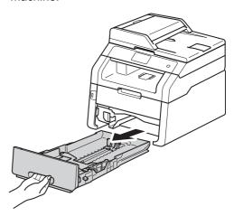
While pressing the green paper-guide release lever ①, slide the paper guides to fit the paper size you are loading in the tray. Make sure the guides are firmly in the slots.
