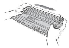
Slide all four drum and toner cartridge assemblies into the machine. Make sure the toner cartridge colour matches the same colour label on the machine.
