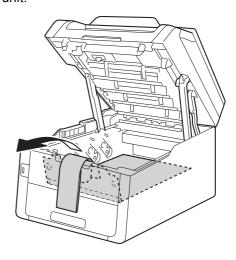
Remove the orange packing piece from each drum and toner cartridge assembly.
