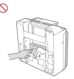
DO NOT carry the machine by holding the scanner cover, the Jam Clear Cover, or the control panel. Doing this may cause the machine to slip out of your hands and may result in injury. Only carry the machine by placing your hands under the entire machine.
