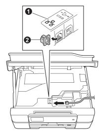
Carefully guide the network cable into the cable channel and out the back of the machine. Connect the cable to your network.
