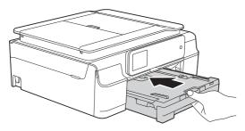
While holding the paper tray in place, pull out the paper support ① until it clicks, and then unfold the paper support flap ②.
