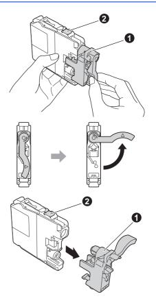
Take care to match the sticker colour **1** with the cartridge colour **2** as shown in the diagram below.
