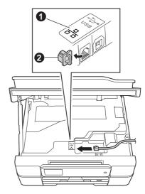
Carefully guide the network cable into the cable channel and out the back of the machine.
