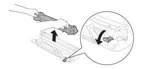
8 Put the toner cartridge back into the drum unit until the lock lever lifts automatically.
