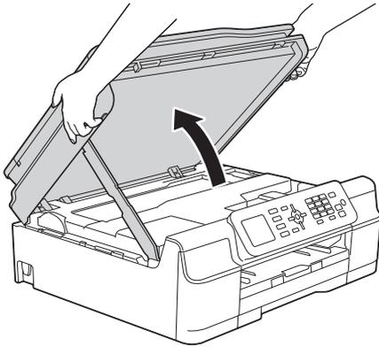
**b** Connect the USB cable to the USB port marked with a
