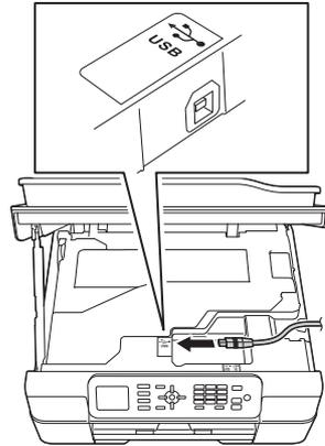
**c** Carefully guide the USB cable into the cable channel and out the back of the machine. Connect the cable to your Macintosh.
