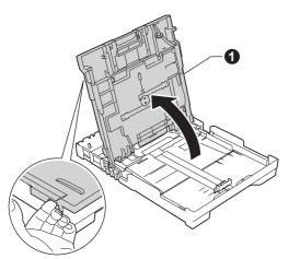
C Gently press and slide the paper width guides ● and then the paper length guide ② to fit the paper size.
