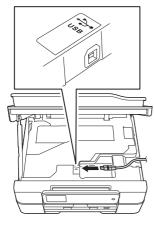
C Carefully guide the USB cable into the cable channel and out the back of the machine. Connect the cable to your computer.
