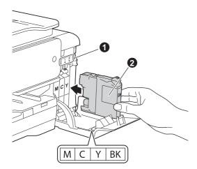
Gently push the back of the ink cartridge marked "PUSH" until the cartridge lever lifts. After all the ink cartridges are installed, close the ink cartridge cover.
