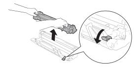
8 Put the toner cartridge back into the drum unit until the lock lever lifts automatically.
