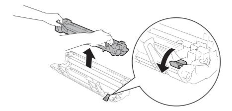
Turn the drum unit gear by hand while looking at the surface of the drum roller (1).
