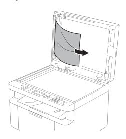
6 Insert a piece of stiff paper, such as cardstock, into the ADF to push any small paper scraps through.
