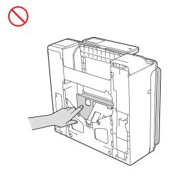
DO NOT carry the machine by holding the scanner cover, the Jam Clear Cover or control panel. Doing so may cause the machine to slip out of your hands. Only carry the machine by placing your hands under the entire machine.
