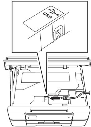
**c** Carefully guide the USB cable into the cable channel and out the back of the machine. Connect the cable to your Macintosh.
