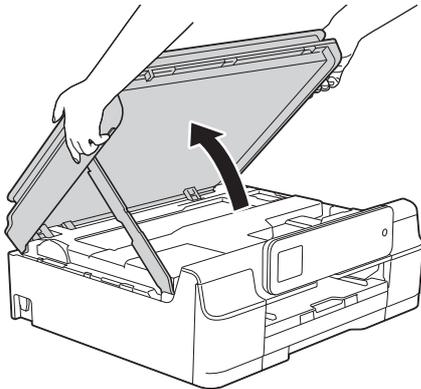
**b** Connect the USB cable to the USB port marked with a
