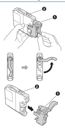
Take care to match the sticker colour **1** with the cartridge colour **2** as shown in the diagram below.
