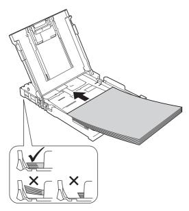
Gently adjust the paper width guides to the paper with both hands. Make sure that the paper width guides touch the edges of the paper.
