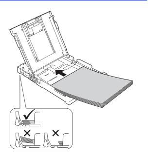
Gently adjust the paper width guides to the paper with both hands. Make sure that the paper width guides touch the edges of the paper.
