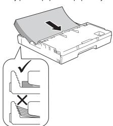
Gently adjust the paper side guides to fit the paper with both hands. Make sure that the paper side guides touch the sides of the paper.
