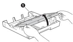
Gently press and slide the paper length guide 1 to fit the paper size.
