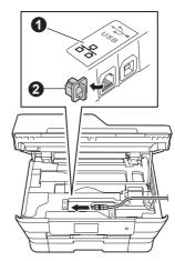
Carefully guide the network cable into the cable channel and out the back of the machine.
