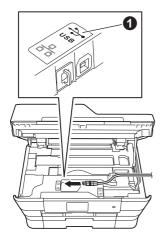
Carefully guide the USB cable into the cable channel and out the back of the machine.
