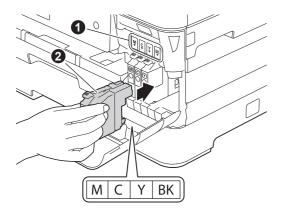
Gently push the back of the ink cartridge marked "PUSH" until the cartridge lever lifts. After all the ink cartridges are installed, close the ink cartridge cover.
