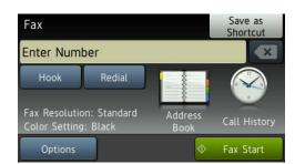
You can change the following fax-sending settings. Press Options. Swipe up or down, or press ▲ or ▼ to scroll through the fax settings. When the setting you want is displayed, press it and choose your new option. When you are finished changing the options, press OK.
