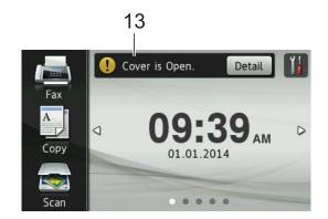
The warning icon ! appears when there is an error or maintenance message; press Detail to view it, and then press to return to Ready mode.
