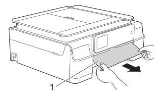
5 Lift the Jam Clear Flap, and remove the jammed paper.
