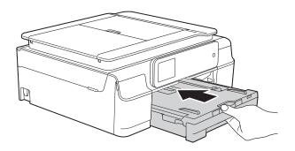
While holding the paper tray in place, pull out the paper support (1) until it locks into place, and then unfold the paper support flap (2).
