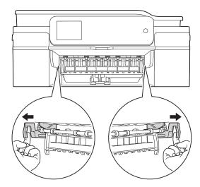
4 Place both hands under the plastic tabs on both sides of the machine to lift the scanner cover into the open position.
