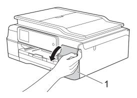
Press the lock release lever as shown to release the cartridge indicated on the Touchscreen. Remove the cartridge from the machine.
