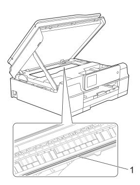
If the paper is jammed under the print head, unplug the machine from the power source, and then move the print head to take out the paper. If the print head is in the right corner as shown in the illustration, you cannot move it. Re-connect the power cord. Hold down until the print head moves to the centre. Then unplug the machine from the power source and take out the paper.
