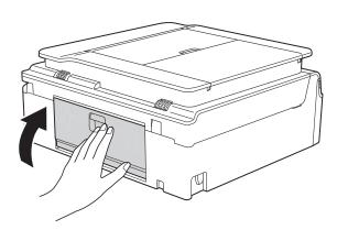
Place both hands under the plastic tabs on both sides of the machine to lift the scanner cover (1) into the open position. Move the print head (if necessary) to take out any paper remaining in this area. Make sure that jammed paper is not left in the corners of the machine (2) and (3).
