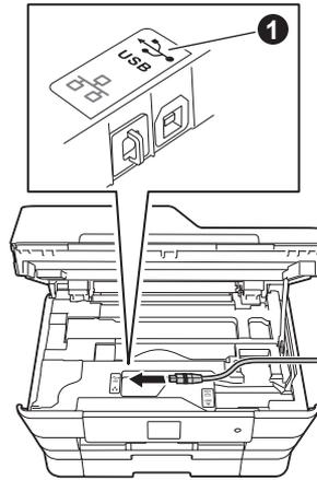
**c** Carefully guide the USB cable into the cable channel and out the back of the machine. Connect the cable to your Macintosh.
