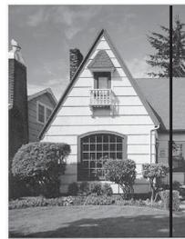
When there is a spot of dirt or correction fluid on the glass strip, the printed sample displays a vertical line.
