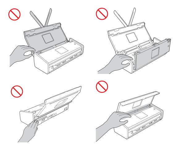
Be careful when touching the Separation Pad and its surrounding area in the machine. Otherwise, you could cause injury to yourself, and serious damage to the machine.
