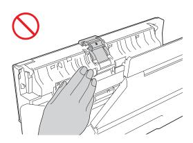
DO NOT carry the machine by holding the top cover. Doing this may cause the machine to slip out of your hands. Only carry the machine by placing your hands under the entire machine.
