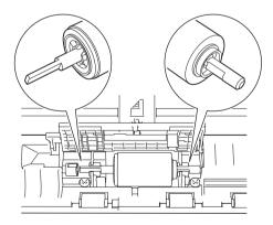
10 Slide the Pick-up Roller (1) to the left edge while turning the Pick-up Roller.
