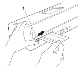
3 Insert the plastic card into the Card Slot (1). The card will be fed into the machine.
