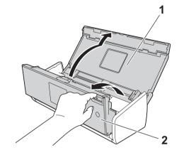
3 In the document feeder unit, clean the glass strips (1) (2) with a soft lint-free cloth moistened with water.
