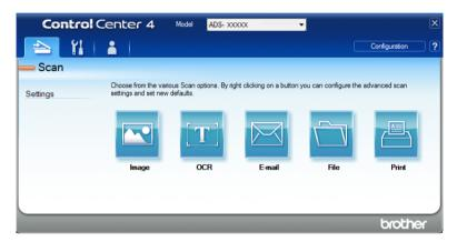
Click **Configuration** and then select **Create custom tab**. You can also create a custom tab by rightclicking the tab area and selecting **Create custom tab**. A custom tab will be created.
