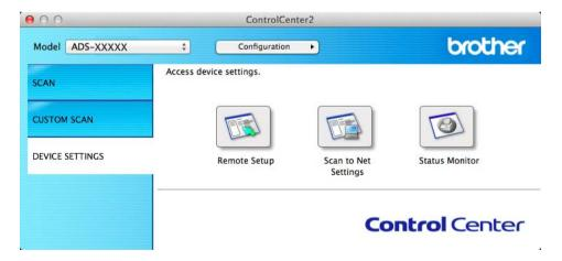
2 Click the **Remote Setup** button. The Remote Setup window will appear.
