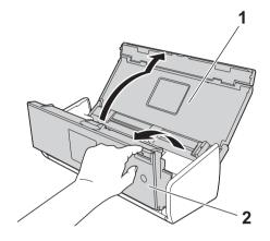
Pinch the Pick-up Roller Cover (1) and then pull the cover up. 2
