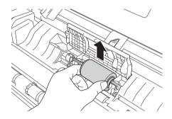
6 Place a new Pick-up Roller into the machine.
