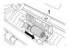
4 The holder of the Pick-up Roller has a narrow opening, and the shape of the shaft of the Pick-up Roller matches this opening. Rotate the Pick-up Roller until you can fit the shaft into the opening of the holder.
