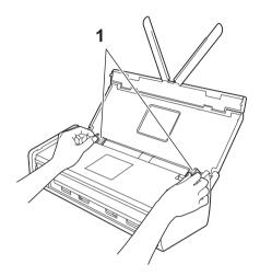
3 Place the Receipt Carrier Sheet in the document feeder between the Guides until you feel it touch the inside of the machine.
