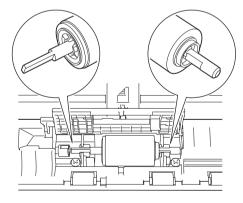
Slide the Pick-up Roller (1) to the left edge while turning the Pick-up Roller.
