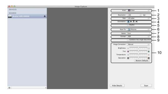
You can adjust the following settings, if needed, in the dialog box accessed by clicking on **Show Details**. Note that the item name and assignable value will vary depending on the machine.
