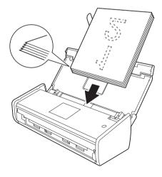
6 Make sure that the side edges of the document are parallel to the grooves in the Top Cover, and then adjust the Guides to fit the width of the document again.
