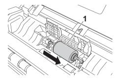
6 The holder of the Pick-up Roller has a narrow opening that is designed to avoid dropping the roller, and the shape of the shaft of the Pick-up Roller matches the opening. Turn the Pick-up Roller around until the shape of the shaft matches the opening of the holder.
