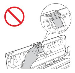
Output the Separation Pad upward.
