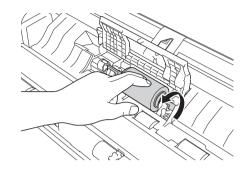
Pinch and pull the Pick-up Roller out of the machine.
