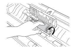
5 Pinch and pull the Pick-up Roller out of the machine.
