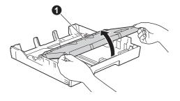
Gently press and slide the paper length guide 1 to fit the paper size.
