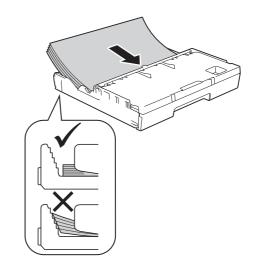
**h** Gently adjust the paper side guides to fit the paper with both hands. Make sure that the paper side guides touch the sides of the paper.
