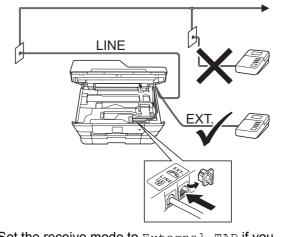
Set the receive mode to External TAD if you have an external answering machine. See Choose a Receive Mode on page 10. Detailed information ➤>Basic User's Guide: Connecting an external TAD (telephone answering device)
