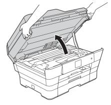
Store the orange protective part in the holder inside the machine as shown.
