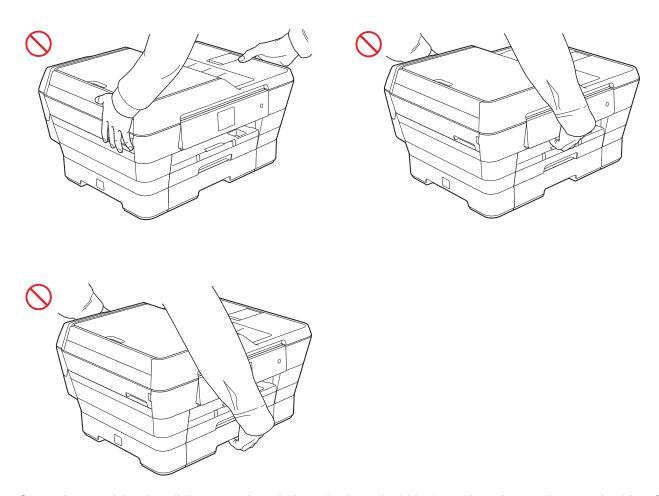
Carry the machine by sliding your hands into the handhold indentations located on each side of the machine.
