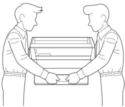
DO NOT carry the machine by holding the scanner cover, the Jam Clear Cover, manual feed slot cover or control panel. Doing so may cause the machine to slip out of your hands.
