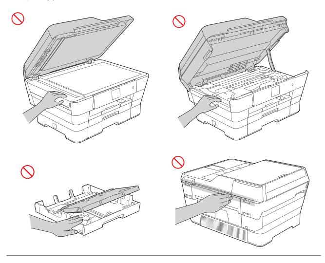
When adjusting the tray size from A3, Legal or Ledger to the original size, take care not to pinch your fingers in the gaps or slots at the bottom of the tray to avoid injury.
