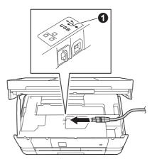
Carefully guide the USB cable into the cable channel and out the back of the machine.
