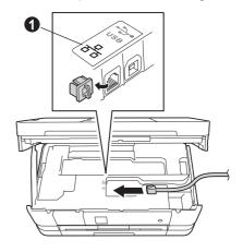
Carefully guide the network cable into the cable channel and out the back of the machine.
