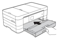
While holding the paper tray in place, pull out the paper support ① until it clicks, and then unfold the paper support flap ②.
