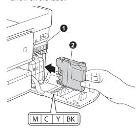
Gently push the back of the ink cartridge marked "PUSH" until it latches. After all the ink cartridges are installed close the ink cartridge cover.
