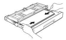
Check that the paper is flat in the tray and below the maximum paper mark ①. Close the output paper tray cover.
