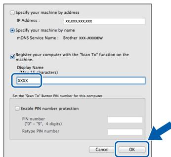
If you want to use the scan feature directly from your machine to scan over the network, you must check the **Register your computer with the "Scan To" function on the machine box**. Click **OK**. Go to **f**.
