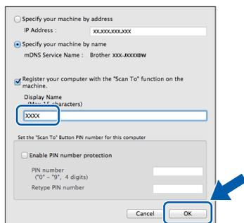
If you want to use the scan feature directly from your machine to scan over the network, you must check the **Register your computer with the "Scan To" function on the machine box**. Click **OK**. Go to **g**.
