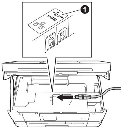
**c** Carefully guide the USB cable into the cable channel and out the back of the machine. Connect the cable to your computer.
