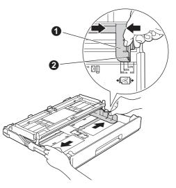
Fan the stack of paper well to avoid paper jams and misfeeds.
