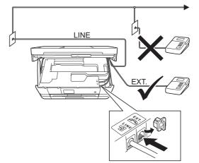
Set the receive mode to External TAD if you have an external answering machine. See Choose a Receive Mode on page 9. Detailed information ➤>Basic User's Guide: Connecting an external TAD (telephone answering device)
