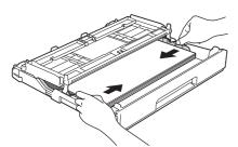
G Check that the paper is flat in the tray and below the maximum paper mark ●. Close the output paper tray cover.
