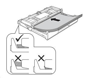
Gently adjust the paper guides to fit the paper. Make sure that the paper guides touch the edges of the paper.
