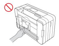
DO NOT carry the machine by holding the scanner cover, the Jam Clear Cover, manual feed slot cover or control panel. Doing so may cause the machine to slip out of your hands. Carry the machine by sliding your hands into the handhold indentations located on each side of the machine.
