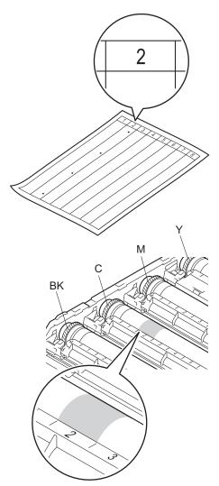
Once the drum has been selected, place one hand on the drum gear and at the other end of that drum place your other hand on the edge, then rotate the drum slowly towards you while looking at the surface of the suspected area.
