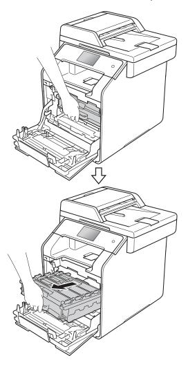
4 Turn the blue lock lever (1) at the left of the machine counterclockwise to the release position. Holding the blue handles of the drum unit, lift the front of the drum unit and remove it from the machine.
