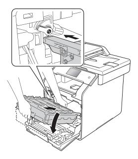
7 Turn the blue lock lever (1) clockwise to the lock position.
