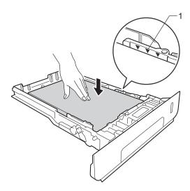
Dut the paper tray *firmly* back in the machine. Make sure the tray is completely inserted into the machine.
