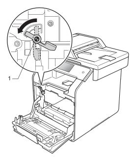
Gently slide the drum unit into the machine until it stops at the blue lock lever.
