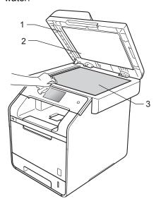
In the ADF unit, clean the white bar (1) and the scanner glass strip (2) underneath it with a soft lint-free cloth gently moistened with water.
