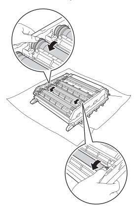
When you have found the mark on the drum that matches the drum dot check sheet, wipe the surface of the drum gently with a cotton swab until the mark on the surface comes off.
