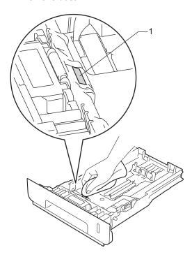
6 Wipe the two pick-up rollers (1) inside the machine to remove dust.
