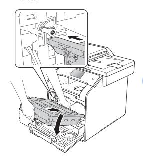
Turn the blue lock lever (1) clockwise to the lock position.
