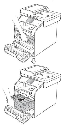
4 Hold the handle of the toner cartridge and gently push it toward the machine to unlock it. Then pull it out of the drum unit. Repeat this for all the toner cartridges.
