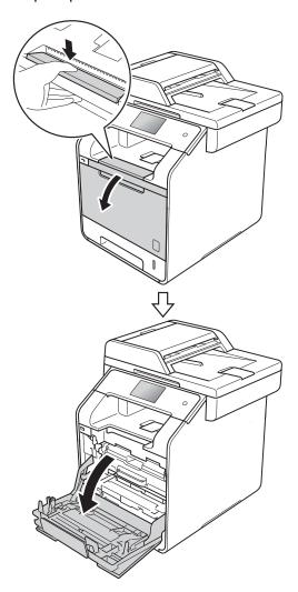
Hold the blue handle of the drum unit. Pull the drum unit out until it stops.
