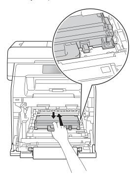
Slide the belt unit back into the machine. Make sure the belt unit is level and fits firmly into place.
