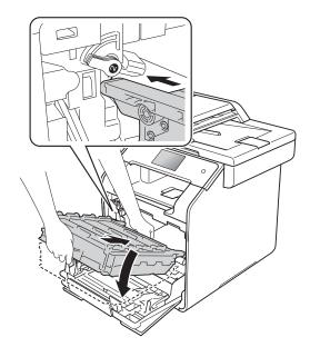
9 Turn the blue lock lever (1) clockwise to the lock position.
