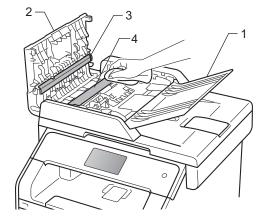
3 Lift the document cover (1). Clean the white plastic surface (2) and scanner glass (3) underneath it with a soft lint-free cloth gently moistened with water.
