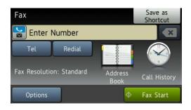
3 To change fax sending settings, press Options. Swipe up or down, or press ▲ or ▼ to scroll through the fax settings. When the setting you want is displayed, press it and choose your new option. When you have finished changing the options, press OK.
