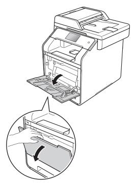
Pull out the MP tray support (1) and unfold the flap (2).
