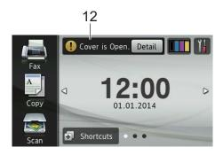
The warning icon ! appears when there is an error or maintenance message; press Detail to view it, and then press
