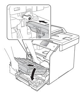
Turn the blue lock lever (1) clockwise to the lock position.
