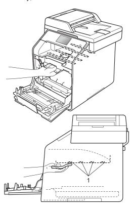
6 Make sure the blue lock lever (1) is in the release position as shown in the illustration.
