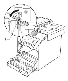
7 Gently slide the drum unit into the machine until it stops at the blue lock lever.
