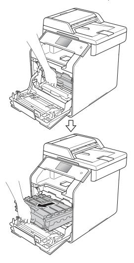
Turn the blue lock lever (1) at the left of the machine counterclockwise to the release position. Holding the blue handles of the drum unit, lift the front of the drum unit and remove it from the machine.
