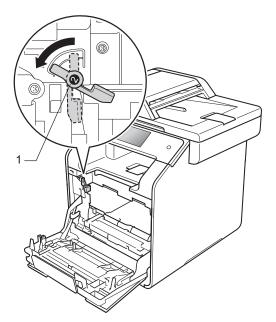
8 Gently slide the drum unit into the machine until it stops at the blue lock lever.
