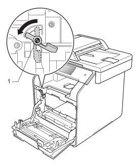
(1) Gently slide the drum unit into the machine until it stops at the blue lock lever.
