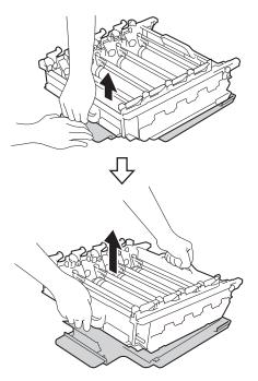
7 Hold the handle of the toner cartridge and slide it into the appropriate colored section of the drum unit until it clicks into place.
