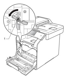
6 Gently slide the drum unit into the machine until it stops at the blue lock lever.
