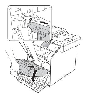
10 Turn the blue lock lever (1) clockwise to the lock position.
