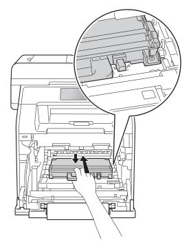
Slide the belt unit back into the machine. Make sure the belt unit is level and fits firmly into place.
