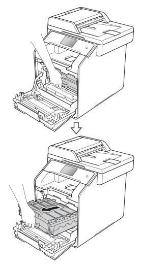
3 Turn the blue lock lever (1) at the left of the machine counterclockwise to the release position. Holding the blue handles of the drum unit, lift the front of the drum unit and remove it from the machine.
