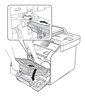
12 Turn the blue lock lever (1) clockwise to the lock position.
