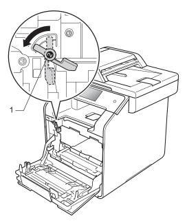
9 Gently slide the drum unit into the machine until it stops at the blue lock lever.
