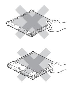
6 Unpack the new belt unit and install the new belt unit in the machine. Make sure the belt unit is level and fits firmly into place.
