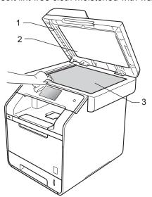
In the ADF unit, clean the white bar (1) and the scanner glass strip (2) underneath it with a soft lint-free cloth moistened with water. Read the NOTE and go to step <sup>(5)</sup>
