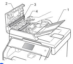
3 Lift the document cover (1). Clean the white plastic surface (2) and scanner glass (3) underneath it with a soft lint-free cloth moistened with water.
