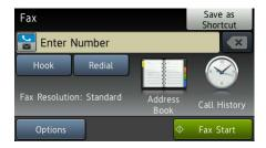
3 To change fax sending settings, press Options. Swipe up or down, or press ▲ or ▼ to scroll through the fax settings. When the setting you want is displayed, press it and choose your new option. When you have finished changing the options, press OK.
