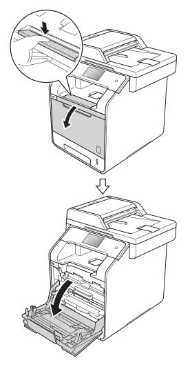
3 Hold the blue handle of the drum unit. Pull the drum unit out until it stops.
