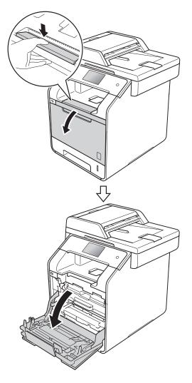
2 Hold the blue handle of the drum unit. Pull the drum unit out until it stops.
