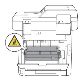
3 Pull the blue tabs (1) at the left and right sides toward you to release the fuser cover (2).
