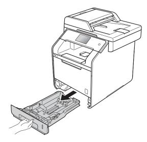
2 While pressing the blue paper-guide release levers (1), slide the paper guides to fit the paper you are loading in the tray. Make sure the guides are firmly in the slots.
