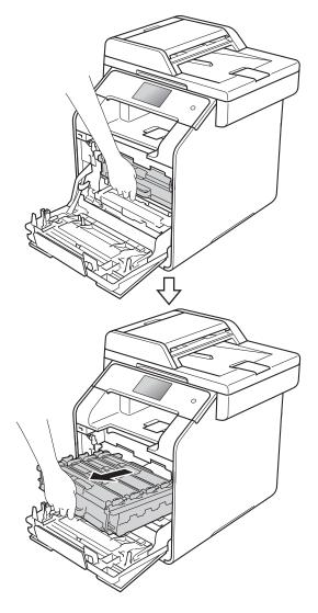
4 Hold the handle of the toner cartridge and gently push it toward the machine to unlock it. Then pull it out of the drum unit. Repeat this for all the toner cartridges.
