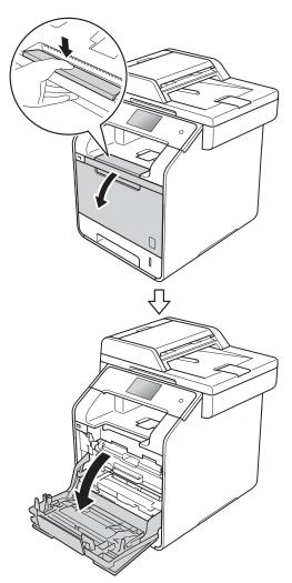
3 Hold the blue handle of the drum unit. Pull the drum unit out until it stops.
