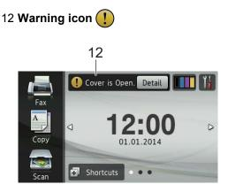
The warning icon (!) appears when there is an error or maintenance message; press Detail to view it, and then press
