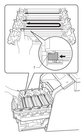
6 Repeat step **5** to clean each of three remaining corona wires.
