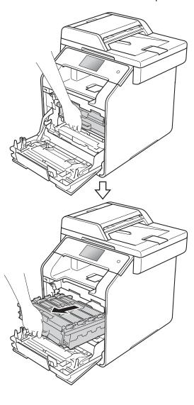
4 Hold the handle of the toner cartridge and gently push it toward the machine to unlock it. Then pull it out of the drum unit. Repeat this for all the toner cartridges.
