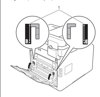
If creases occur with the envelope levers in the envelope position, print with the back cover opened and feed one envelope at a time from the MP tray.
