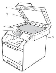
In the ADF unit, clean the white bar (1) and the scanner glass strip (2) underneath it with a soft lint-free cloth moistened with water. Read the NOTE and go to step 6
