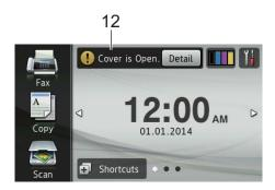
The warning icon papears when there is an error or maintenance message; press Detail to view it, and then press
