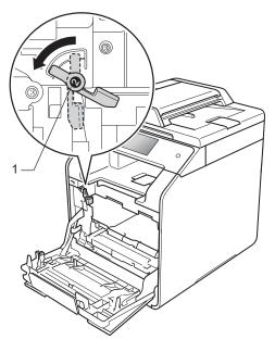
Gently slide the drum unit into the machine until it stops at the blue lock lever.
