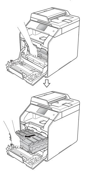
Turn the blue lock lever (1) at the left of the machine counterclockwise to the release position. Holding the blue handles of the drum unit, lift the front of the drum unit and remove it from the machine.
