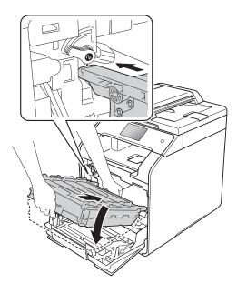
8 Turn the blue lock lever (1) clockwise to the lock position.
