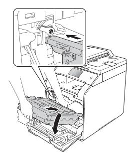
10 Turn the blue lock lever (1) clockwise to the lock position.
