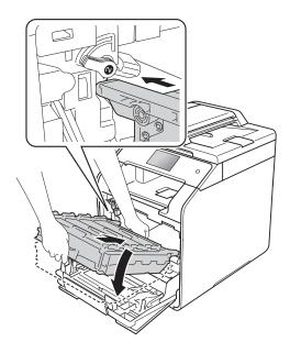
7 Turn the blue lock lever (1) clockwise to the lock position.
