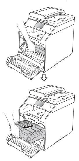
Hold the handle of the toner cartridge and gently push it toward the machine to unlock it. Then pull it out of the drum unit. Repeat this for all the toner cartridges.
