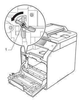
8 Gently slide the drum unit into the machine until it stops at the blue lock lever.
