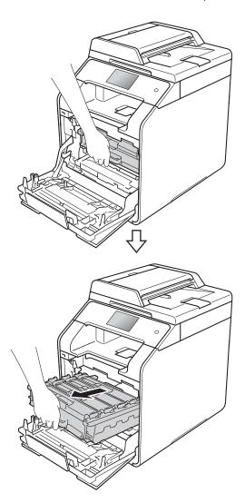
4 Turn the blue lock lever (1) at the left of the machine counterclockwise to the release position. Holding the blue handles of the drum unit, lift the front of the drum unit and remove it from the machine.
