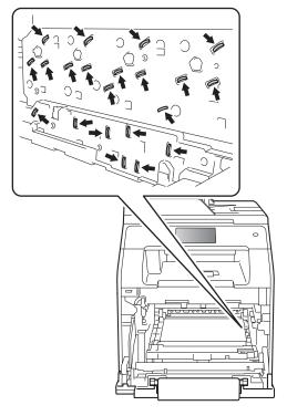
Hold the blue handles of the drum unit when you carry it. DO NOT hold the sides of the drum unit. Wipe the four scanner windows (1) with a dry, lint-free cloth.
