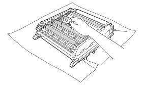
Hold the handle of the toner cartridge and slide the toner cartridge into the drum unit, then gently pull it toward you until you hear it click into place. Make sure that you match the toner cartridge colour to the same colour label on the drum unit. Repeat this for all the toner cartridges.
