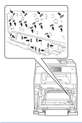
5 Hold the blue handle of the belt unit with both hands and lift the belt unit up, then pull it out.
