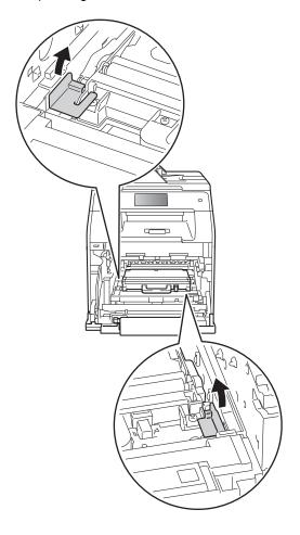
7 Hold the blue handle of the waste toner box and remove the waste toner box from the machine.
