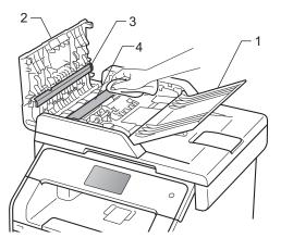
3 Lift the document cover (1). Clean the white plastic surface (2) and scanner glass (3) underneath it with a soft lint-free cloth gently moistened with water.
