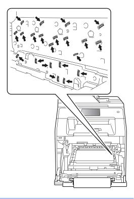
Hold the blue handle of the belt unit with both hands and lift the belt unit up, then pull it out.
