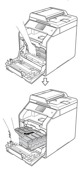
4 Turn the blue lock lever (1) at the left of the machine counterclockwise to the release position. Holding the blue handles of the drum unit, lift the front of the drum unit and remove it from the machine.
