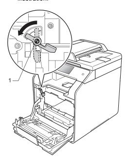
6 Gently slide the drum unit into the machine until it stops at the blue lock lever.
