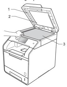
4 In the ADF unit, clean the white bar (1) and the scanner glass strip (2) underneath it with a soft lint-free cloth gently moistened with water.
