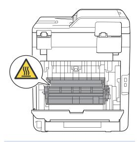
3 Pull the blue tabs (1) at the left and right sides down to release the fuser cover (2).
