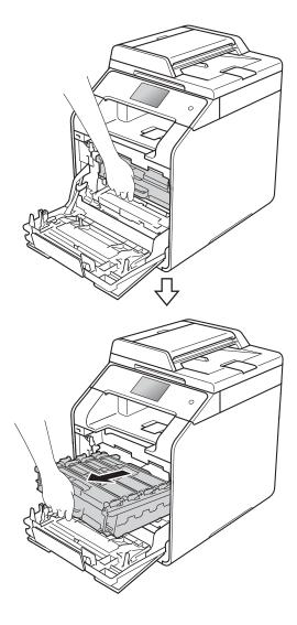
3 Turn the blue lock lever (1) at the left of the machine counterclockwise to the release position. Holding the blue handles of the drum unit, lift the front of the drum unit and remove it from the machine.
