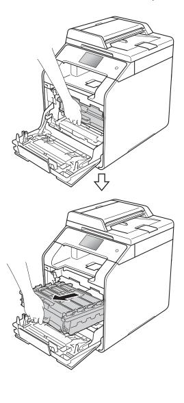
4 Hold the handle of the toner cartridge and gently push it toward the machine to unlock it. Then pull it out of the drum unit. Repeat this for all the toner cartridges.
