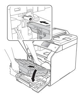
Turn the blue lock lever (1) clockwise to the lock position.
