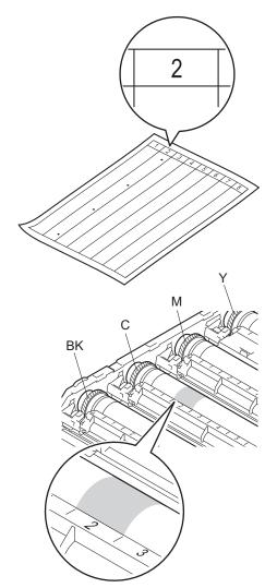
Once the drum has been selected, place one hand on the drum gear and at the other end of that drum place your other hand on the edge, then rotate the drum slowly towards you while looking at the surface of the suspected area.
