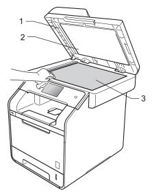
4 In the ADF unit, clean the white bar (1) and the scanner glass strip (2) underneath it with a soft lint-free cloth moistened with water. Read the NOTE and go to step **5**.
