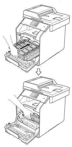
Close the front cover and turn on the machine's power switch.
