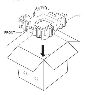
Wrap the machine in a plastic bag, then place it on the bottom packing material (1).
