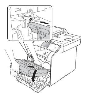
8 Turn the blue lock lever (1) clockwise to the lock position.
