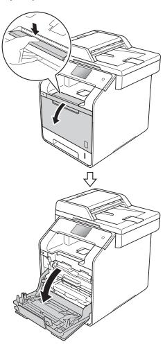
3 Hold the blue handle of the drum unit. Pull the drum unit out until it stops.
