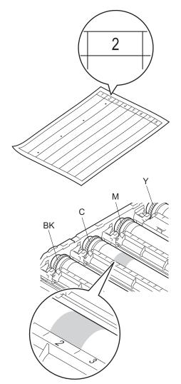
Identify the drum indicated by the colored dot in step . Hold the drum unit frame with both hands, place your left thumb on the drum unit gear, and roll the drum toward you, as illustrated in the drawing below. Look in the numbered area identified in step for any marks or scratches.
