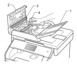
3 Lift the document cover (1). Clean the white plastic surface (2) and scanner glass (3) underneath it with a soft lint-free cloth moistened with water.
