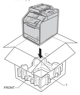
5 Place the packing material (2) marked "RIGHT" on the right of the machine. Place the packing material (3) marked "LEFT" on the left of the machine. Place the AC power cord and printed materials in the original carton as shown in the illustration.
