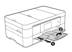
Pull out the paper support 1, and unfold the paper support flap 2
