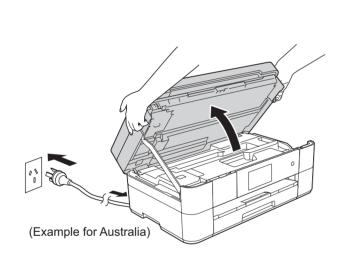
Connect the power cord. Lift the scanner cover.
