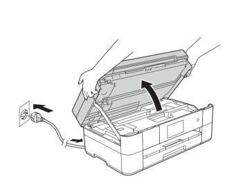
Connect the power cord. Lift the scanner cover.
